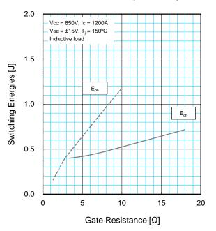
HALF-BRIDGE SWITCHING TIME CHARACTERISTICS (TYPICAL)
